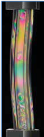
Stress lines show in a transparent I-beam made from an optically active plastic as it is compressed between two crossed polarizers.
