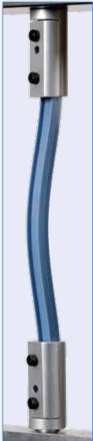
An I-beam from the PASCO Structures System buckles as it is compressed in the Materials Tester.
