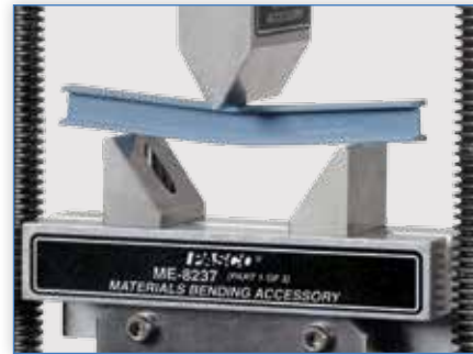
A three-point bending test is performed on a plastic I-beam from the PASCO Structures System.
