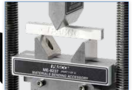
A concrete beam, simulated by pouring plaster of paris into a form with plastic rebar using the PASCO Structures Cast Beam Set, undergoes a bending test.
