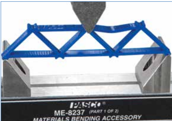
Truss Buckles under Compression in Materials Tester
