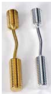
Measure the critical load needed to buckle the sample.
