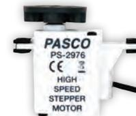
The PASCObot's motion is controlled by two Stepper Motors, which connect to the bot's Wheels. Compatible with other STEM Sense products, the Stepper Motors can be controlled individually to move the bot forwards, backwards, and around corners and curves.
