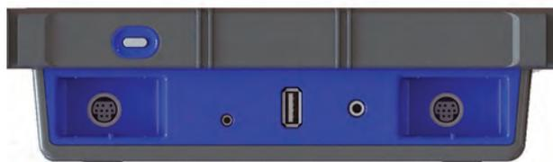
The SPARK LXi2 features two PASPORT ports as well as ports for the included temperature and voltage probes.
